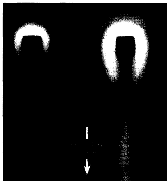
Fig. 2. Developed images from flow tank floor with two parallelepipeds. The observed optical patterns are the result of variations in mass transfer resistance that, in turn, result from the flow field induced by the parallelepipeds.
